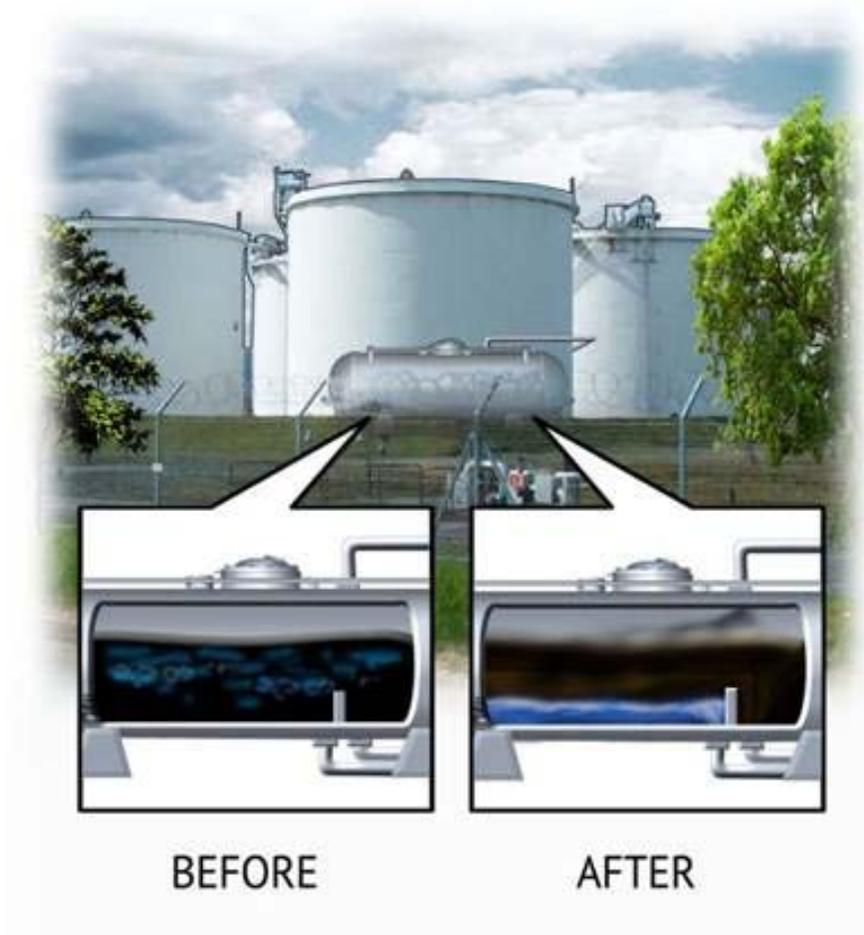
An illustration of how water in a flow station without production additive remains mixed with the crude, causing process slowdowns. Right, the same flow station treated with a low dosage (0.1% to 0.5% by volume) of an incorporative/non-evaporative demulsifying additive that reduces the emulsified water content of the crude to meet refinery standards.
