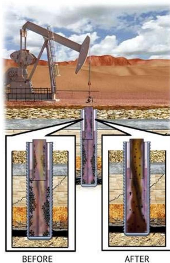
The typical state of an oil well in which no production additives have been used during the extraction phase. Buildup of asphaltene and paraffin in the bore and on the head impede the efficient flow of crude. Right, the same well bore and head as treated with new incorporative/non-evaporative production additives, which can offer improved performance over traditional hexane-based solvents without HSE concerns.
